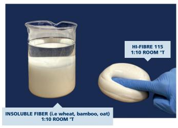
In this picture we show the difference of the water binding properties between a typical insoluble cellulose fiber and Hi-Fibre 115.
